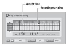
Each row of the grid is one day (you can set the timer recording for up to a month in advance). Each column is a 15 minute interval
